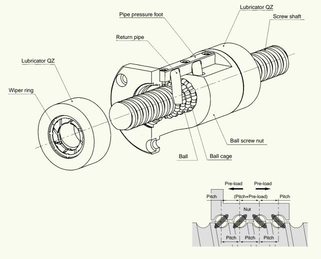
Fig.1 Structure of type SBN
