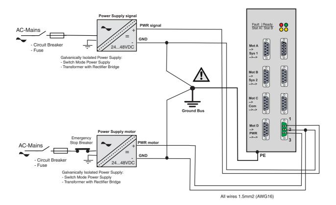
Instead of two separated power supplies it may be possible to use only one power supply if there is no need to control the signal power supply (logical devices of the controller) and the power supply of the powerstage for the motors independently (see safety rules of the application).
