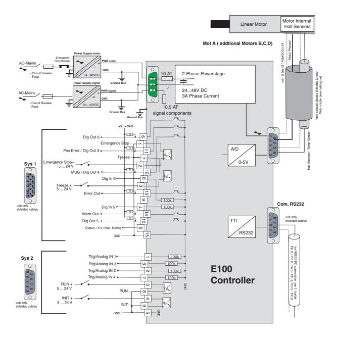
Typical wiring of a single axes controller. Multiple axes controller have additional motor connectors.
