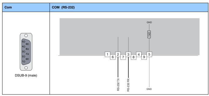
RS232: 9.6kBaud, use 1:1 connection cable to PC
