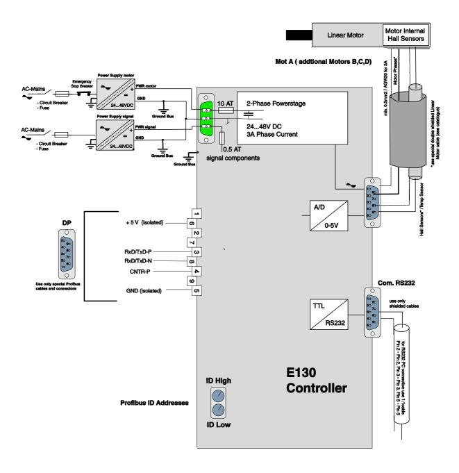
Picture shows typical wiring of a single axes controller. Multiple axes controller will have additional motor connectors.
