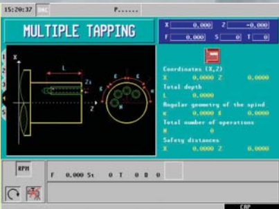
Multiple drilling and tapping
