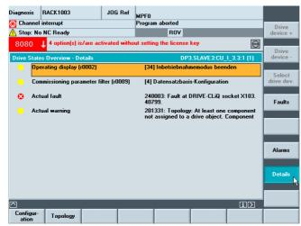
Figure 15-33 "Diagnostics" > "Drive system" > "Details" menu
