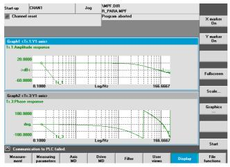
Figure 11-7 Optimized position control loop
