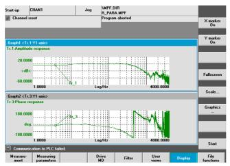
Figure 11-6 Optimized speed control loop
