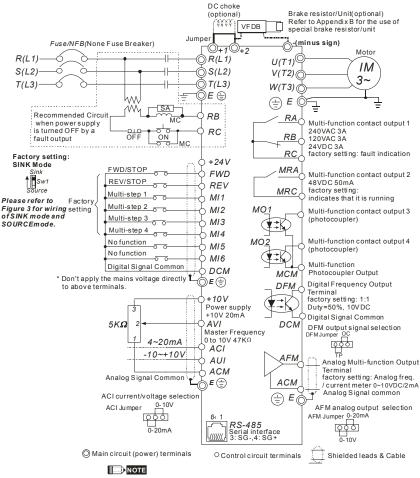
1. Please turn off the power when ACI/DFM/AFM jumpers are inserted/removed.
