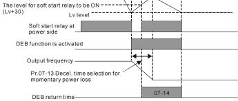
For example, in textile machinery, you will hope that all the machines can be decelerated to stop to prevent broken stitching when power loss. In this case, the host controller will send a message to the AC motor drive to use DEB function with deceleration time via EF.
