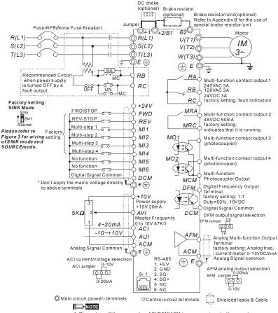
1. Please turn off the power when ACI/DFM/AFM jumpers are inserted/removed.
