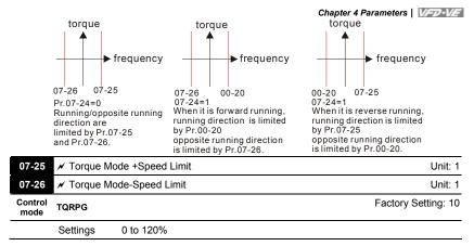
These parameters are used in the torque mode to limit the running direction and opposite
