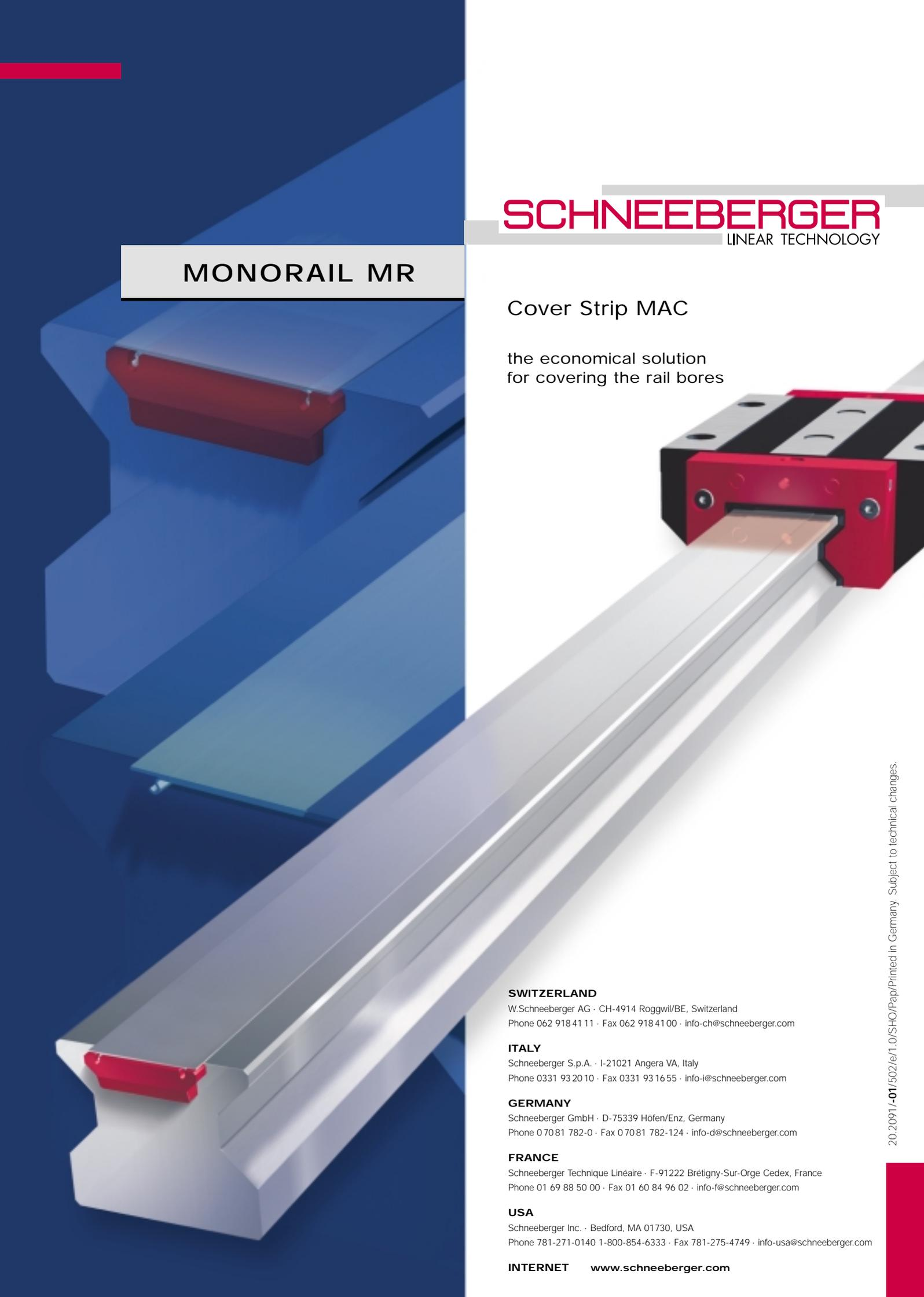
The background features a 3D rendering of a rail assembly. On the left, a blue rail with a red cover strip is shown in a perspective view. On the right, a more detailed view shows a red cover strip being inserted into a groove of a silver rail. The Schneeberger logo is positioned at the top right, with the tagline 'LINEAR TECHNOLOGY' below it.
