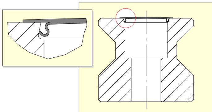
**Robust and clean:** With the design of the legs shaped as a «S» and the undercut groove, the rail cover strip clings tightly to the rail surface. This combination gives a defined wiper surface.
