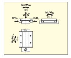
Loading capacities are calculated values, based on DIN 636-2  $C_0$  = static loading capacity C = dynamic loading capacity (100 km)  $M_0$  = static moment M = dynamic moment (100 km)
