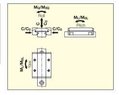
Loading capacities are calculated values, based on DIN 636-2  $C_0$  = static loading capacity C = dynamic loading capacity (100 km)  $M_0$  = static moment M = dynamic moment (100 km)
