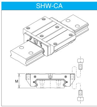
The SHW-CA type features a wide construction and a low center of gravity and can bear load in all 4 directions. The LM block installation holes are tapped and then counterbored from the underside of the flange, allowing the LM block to be mounted from either above or below (fixed at 4 points).
