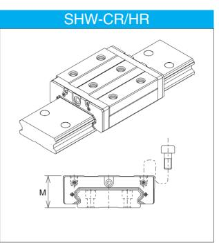
The SHW-CR type is a compact design that features a wide construction and low center of gravity, and can bear loads in all four directions. The LM block is installed using the holes tapped in the upper side. The SHW 12 includes the heavy-load SHW-HR type with an increased rated load capacity. This type features the same cross-sectional profile as the SHW-CR, but with an increased number of balls.
