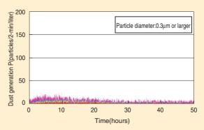
Figure 9 Results of dust generation measurement (using THK AFF grease) for an SHW21CA
