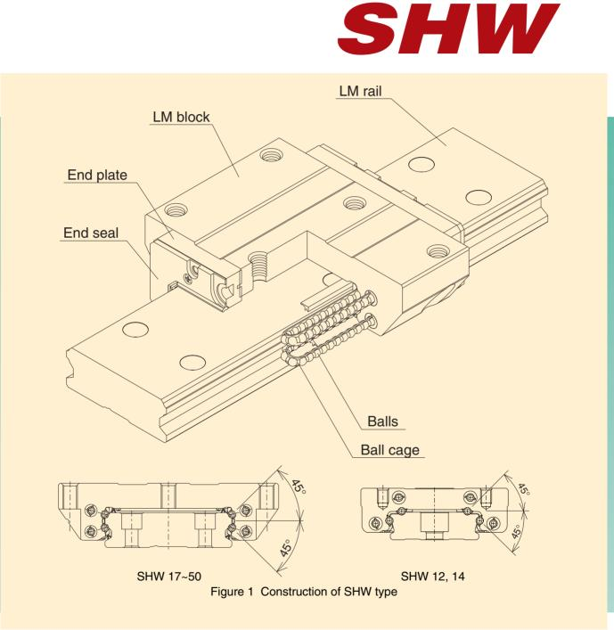
Extra-wide, high-rigidity LM Guide, incorporating Caged Ball<sup>TM</sup> Technology, has been developed to provide users with high speed, low-noise, long-term, maintenance-free service.
