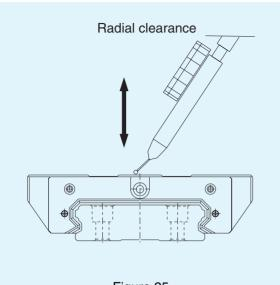
Table 9 shows the radial clearances for SHW-type LM guides. Table 9 Radial clearances for SHW-type LM guides
