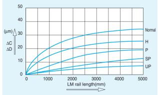
Figure 24 LM rail length and the running parallelism
