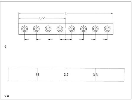
Accuracy of adjacent components An important criterion for the correct performance of a rail guide system is the accuracy of the associated components. The higher the demands for accuracy of guidance and for smooth, easy operation, the greater the attention which must be paid to the accuracy of form and position of the associated components. Generally the same accuracy requirements should be applied to these components as to
