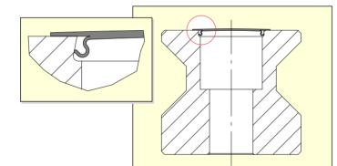
**Robust and clean:** With the design of the legs shaped as a (S) and the undercut groove, the rail cover strip clings tightly to the rail surface. This combination gives a defined wiper surface.
