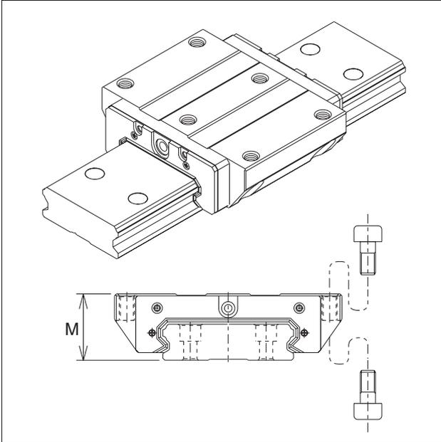
The SHW-CA type features a wide construction and a low center of gravity and can bear load in all 4 directions. The LM block installation holes are tapped and then counterbored from the underside of the flange, allowing the LM block to be mounted from either above or below (fixed at 4 points).
