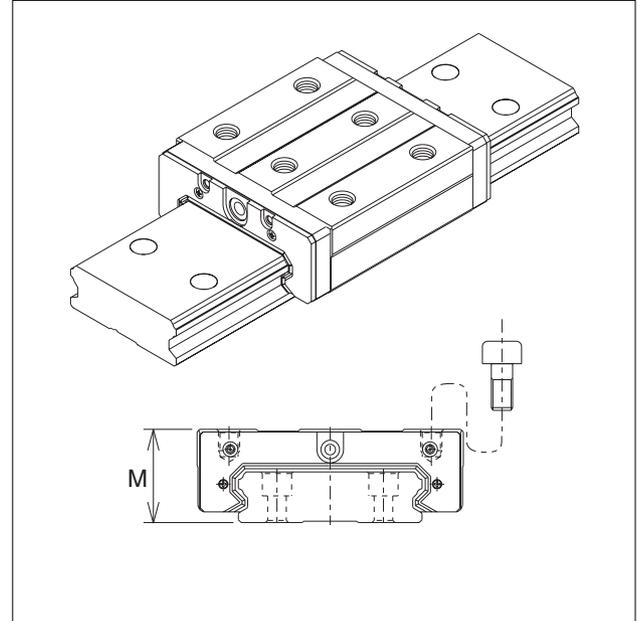
The SHW-CR type is a compact design that features a wide construction and low center of gravity, and can bear loads in all four directions. The LM block is installed using the holes tapped in the upper side. The SHW 12 includes the heavy-load SHW-HR type with an increased rated load capacity. This type features the same cross-sectional profile as the SHW-CR, but with an increased number of balls.
