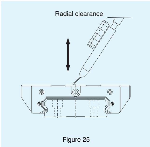
Table 9 shows the radial clearances for SHW-type LM guides.
