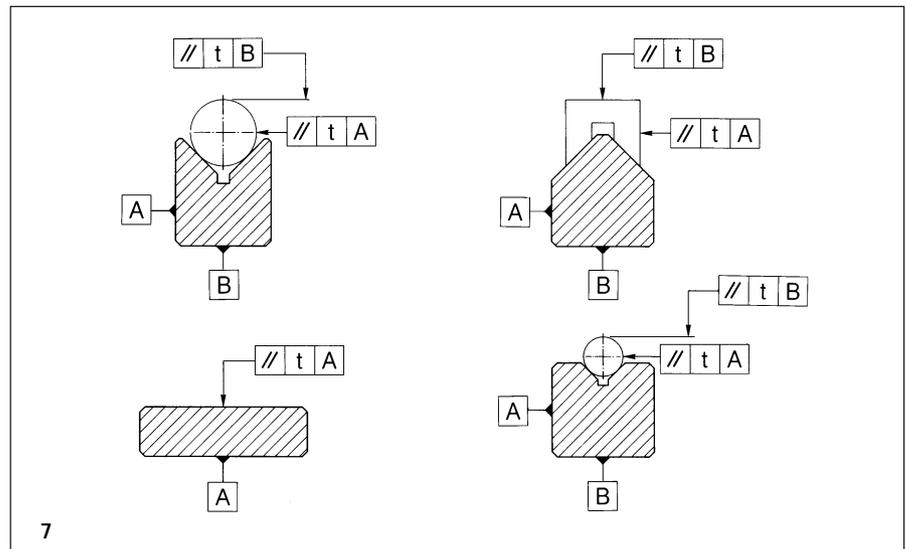
Permissible deviation in parallelism between surfaces A and B
