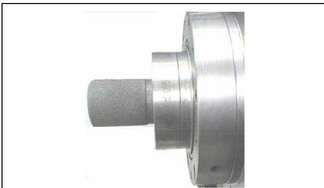
Figure 8.18 use of the gauge as a normal tool-holder, with or without interposed thickness spacer (Figure 8.19), according to the indications of the table shown in the procedures of paragraphs 0 and 0
