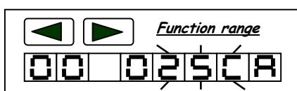
After selection the function you can press **S** key shortly to SAVE its number of line in the program, and also to enter the content register of the function to define its value.
