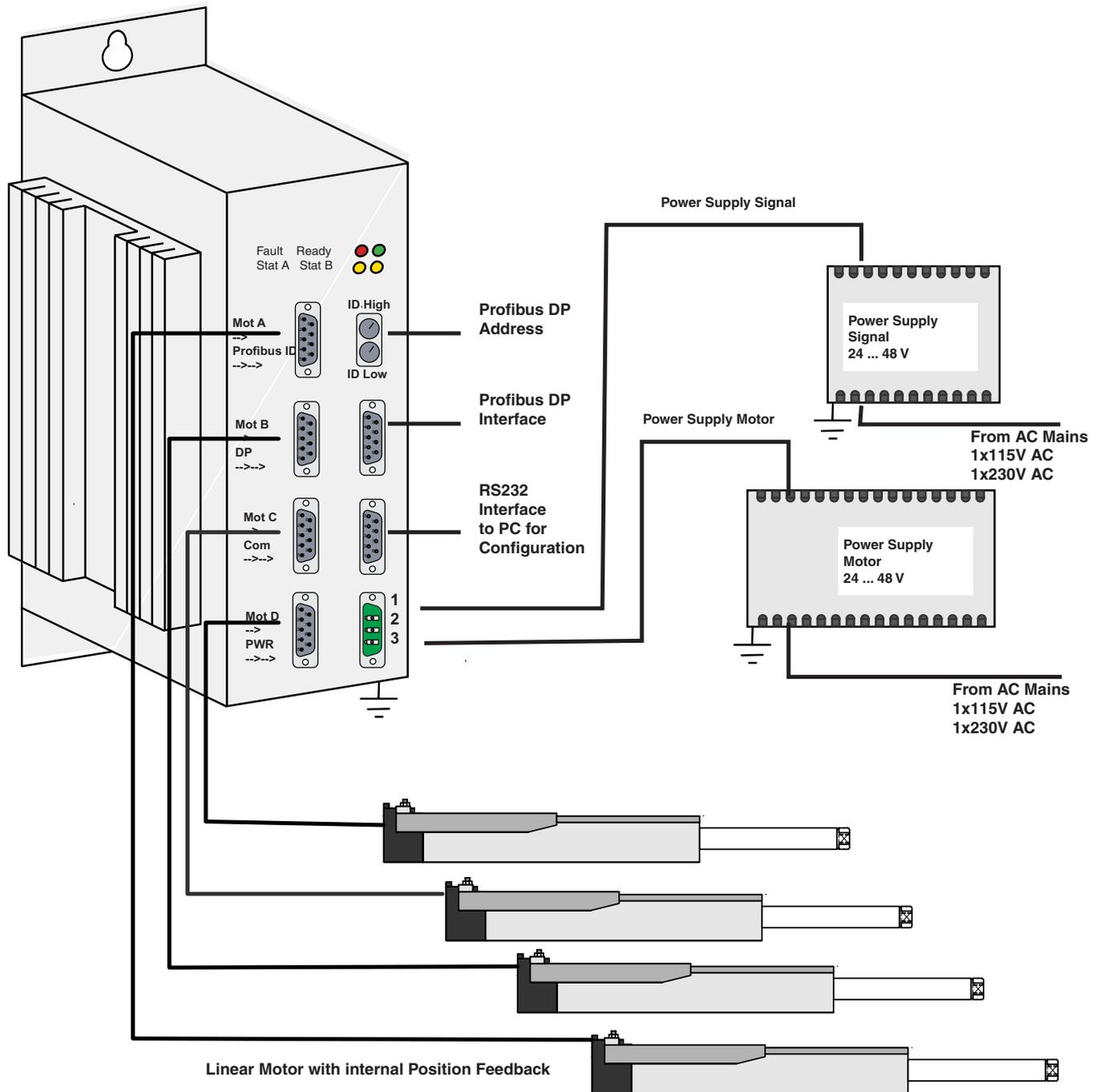
Complete E430 Controller based system (E130 and E230 controllers will only drive one respectively two motors). Power Supply for Signal and Motor may be the same device (see later).
