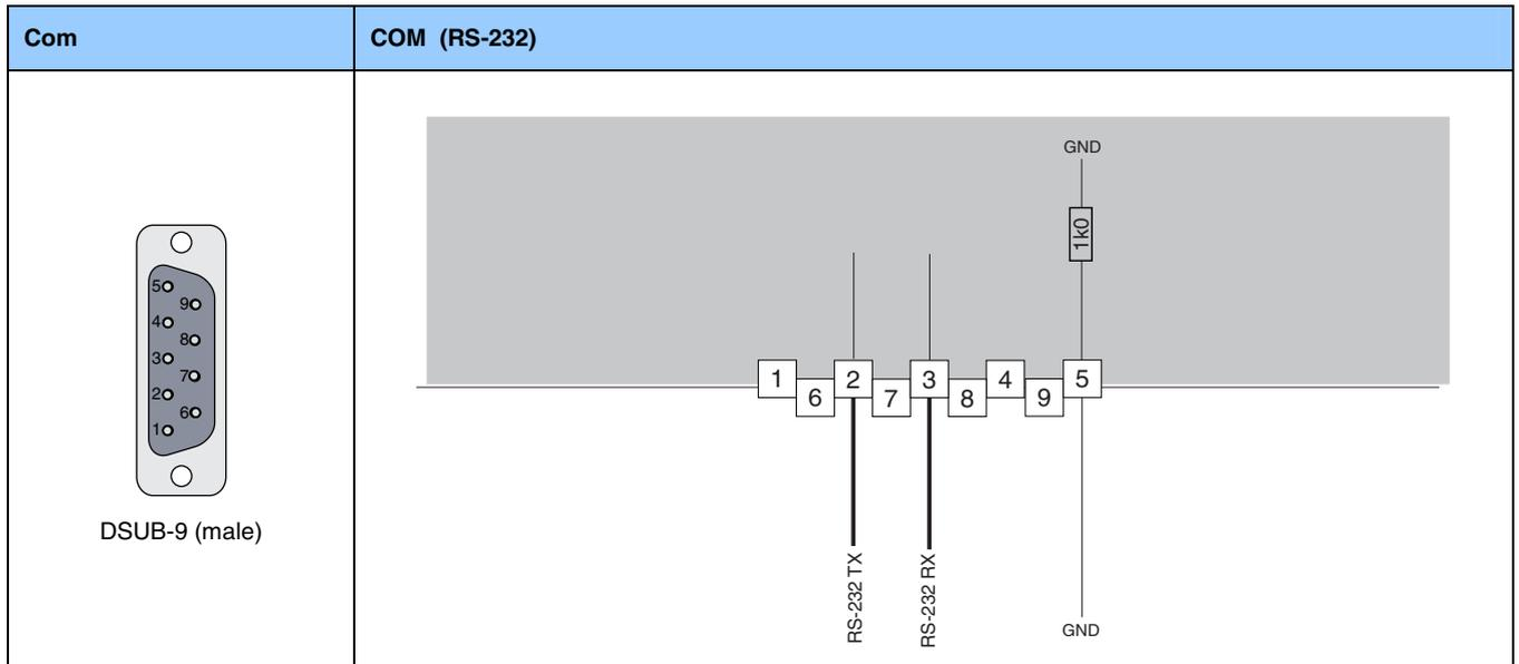
RS232: 9.6kBaud, use 1:1 connection cable to PC
