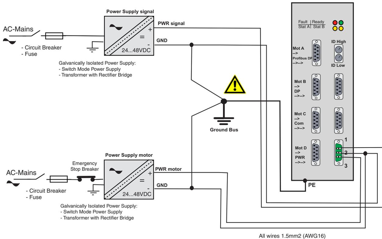
Instead of two separated power supplies it may be possible to use only one power supply if there is no need to control the signal power supply (logical devices of the controller) and the power supply of the powerstage for the motors independently (see safety rules of the application).
