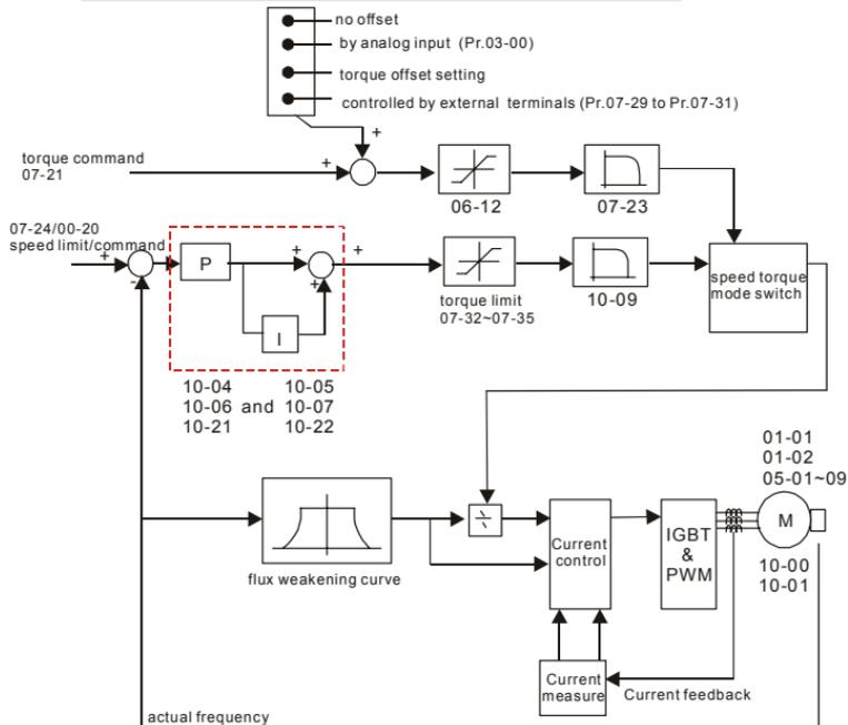
**Control Diagram for the Torque + Encoder**
