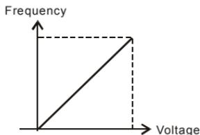
$$F_{\text{command}} = [(ay + \text{bias}) * \text{gain}] * \frac{F_{\text{max}}(01-00)}{10V \text{ or } 16mA}$$
