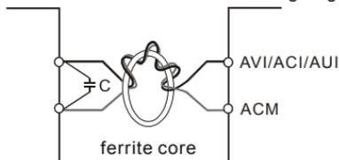
wind each wires 3 times or more around the core
