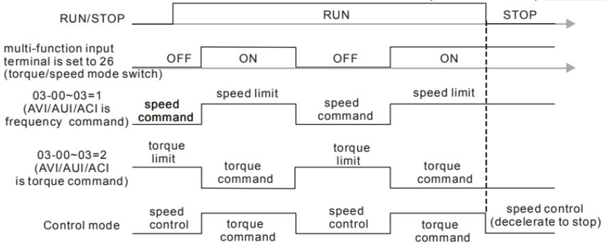
**Torque Control/Speed Control Switch Timing**
