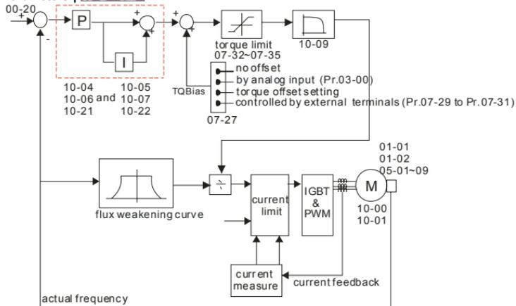
**Control Diagram for the Vector+ Torque**
