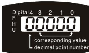
For example, if use rpm to display the motor speed and the corresponding value to the 4-pole motor 60Hz is 1800. This parameter can be set to 01800 to indicate that the corresponding value for 60Hz is 1800rpm. If the unit is rps, it can be set 10300 to indicate the corresponding value for 60Hz is 30.0 (a decimal point).
