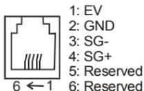
Each VFD-VE AC drive has a pre-assigned communication address specified by Pr.09-00. The RS485 master then controls each AC motor drive according to its communication address.
