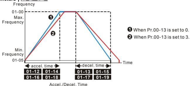
**00-14** Time Unit for Acceleration/Deceleration and S Curve
