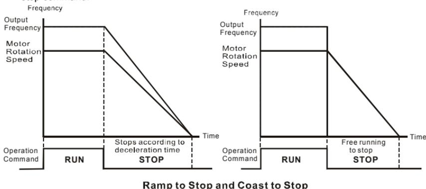
**Ramp to stop:** the AC motor drive decelerates from the maximum output frequency (Pr. 01-00) to minimum output frequency (Pr. 01-09) according to the deceleration time and then stop.
