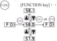
[FUNCTION key] • This key allows the selection of commands and memorises parameters. When the key is pressed once in the state of, the extension function code selection state is set.
