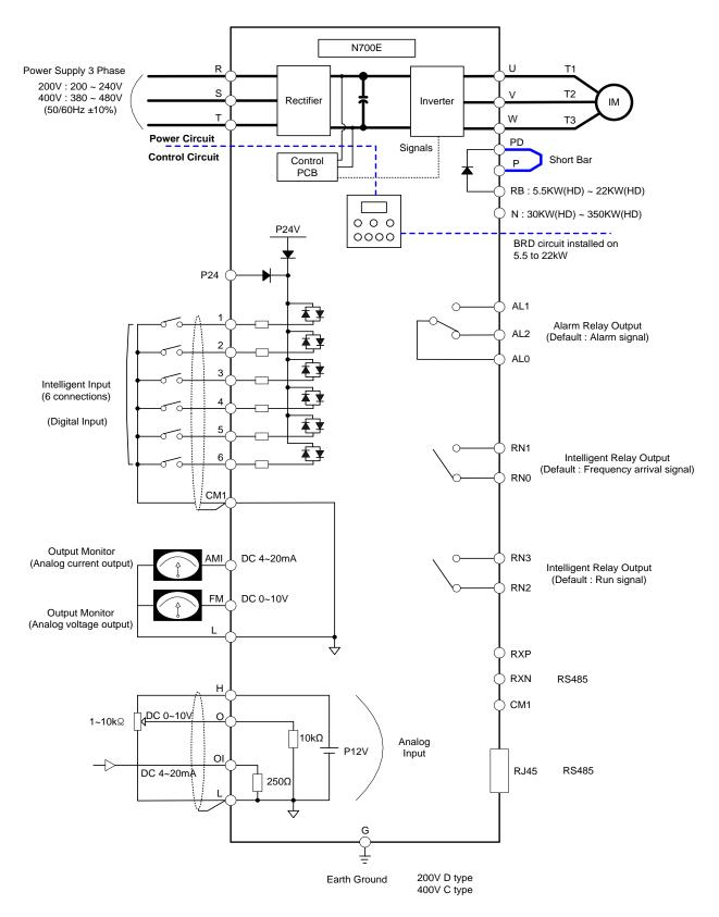
Fig.2-3 Terminal Connection Diagram (sink type)
