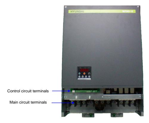
Fig1-6Front cover removed
