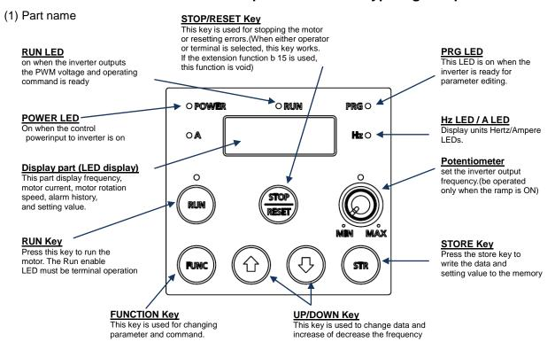
Fig.4-1 LED Type Digital Operator
