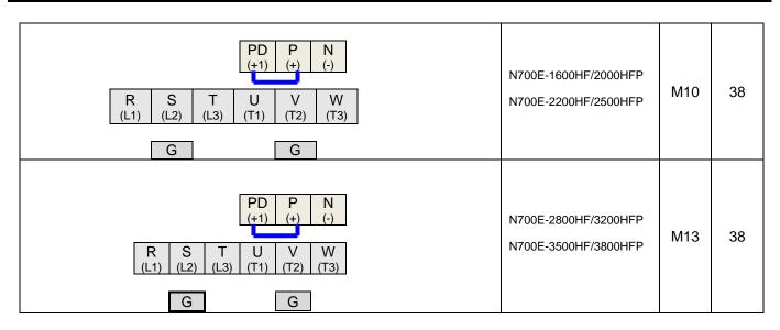
Table 2-3Wiring of main circuit terminals
