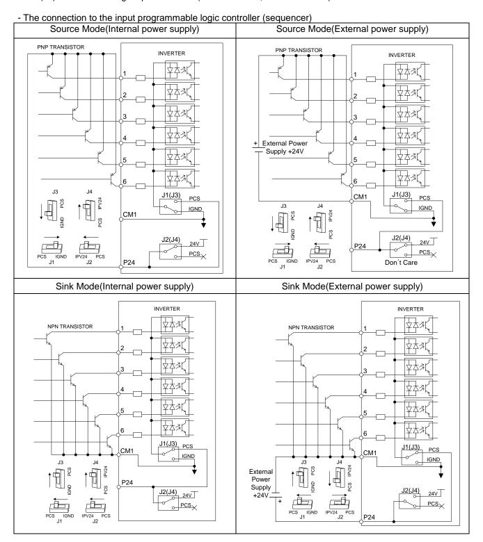
Fig 2-6Input terminal and PLC connection
