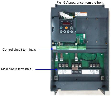
Fig1-4 Front cover removed
