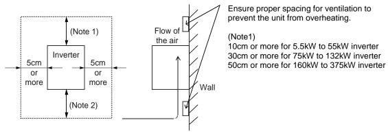
Fig 2- 1Surface for the mounting of inverter
