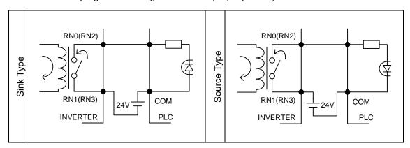
Fig 2-7 Output terminal and PLC connection
