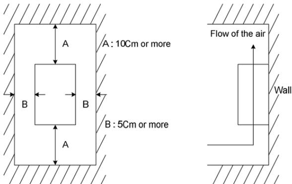
Figure 2-1 Air gap (Installation)
