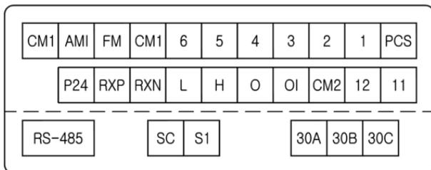
Figure 2-5 Control circuit terminal
