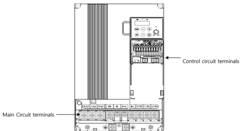
Figure 1-6 Front view without front cover
