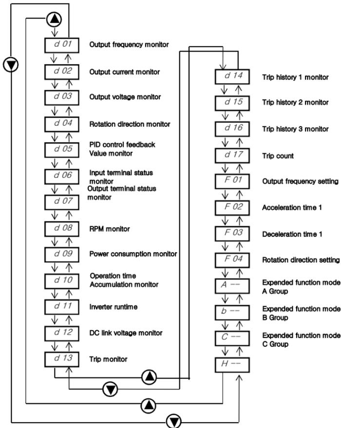
Figure 4-2 Up/Down key basic operation
