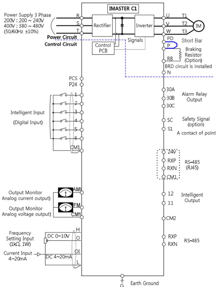
Figure 4-6 Setting diagram from the terminal
