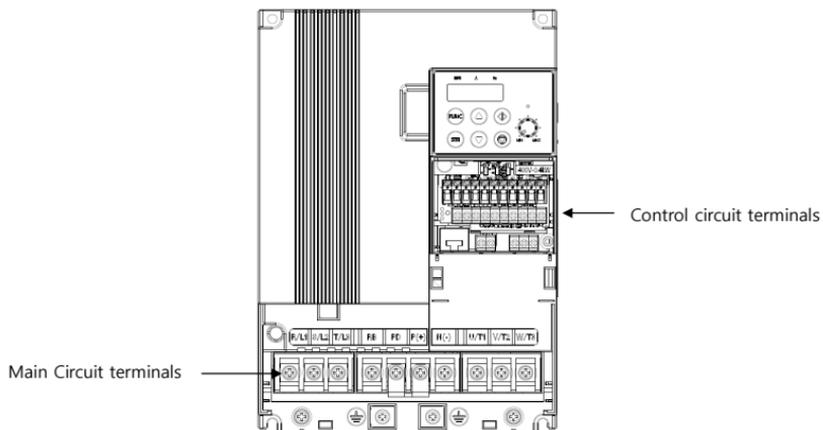
Figure 1-4 Front view without front cover
