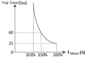
**ij) b05 = 0: Trip Time vs. Motor Current**
