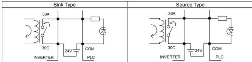
Figure 2-8 Connections between Relay and PLC
