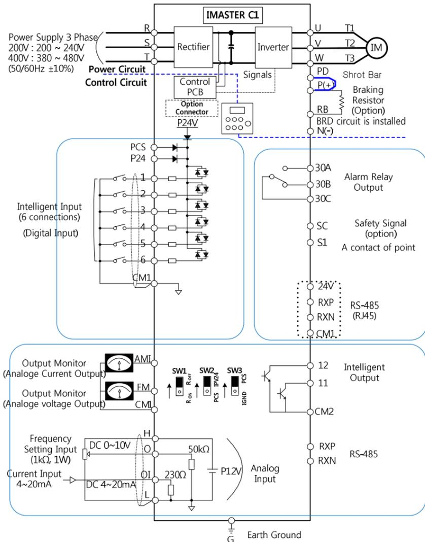
Figure 2-3 Terminal connection diagram (Sink type)
