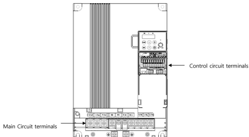
Figure 1-8 Front view without front cover
