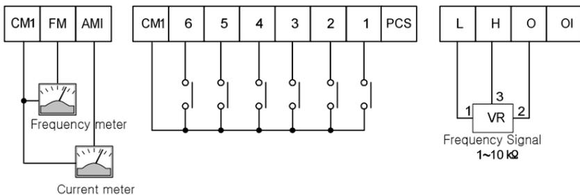
Figure 2-6 Example of control circuit wiring
