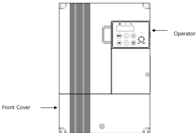
Figure 1-3 Front view with front cover
