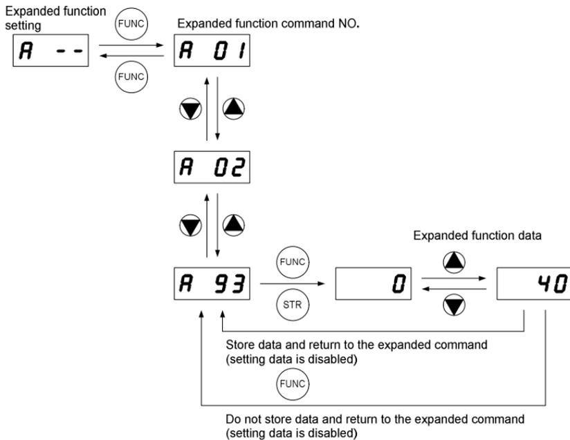
Figure 4-3 Expanded function mode navigation
