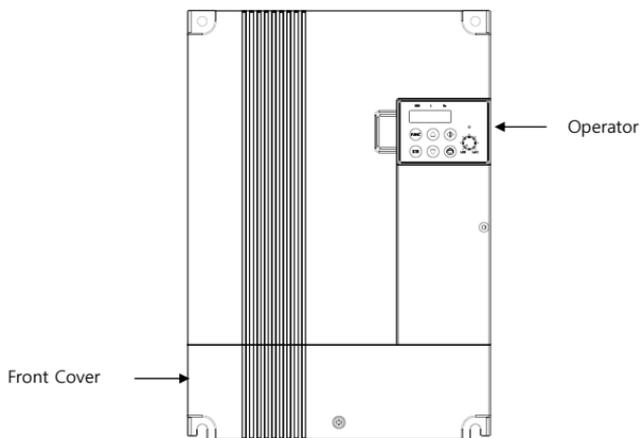
Figure 1-7 Front view with front cover
